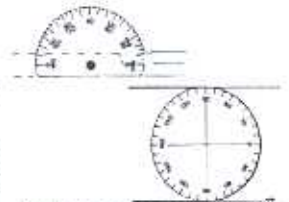
FIGURE 2 - 4. The body of the goniometer can be either a half circle (top) or a full circle (bottom).
