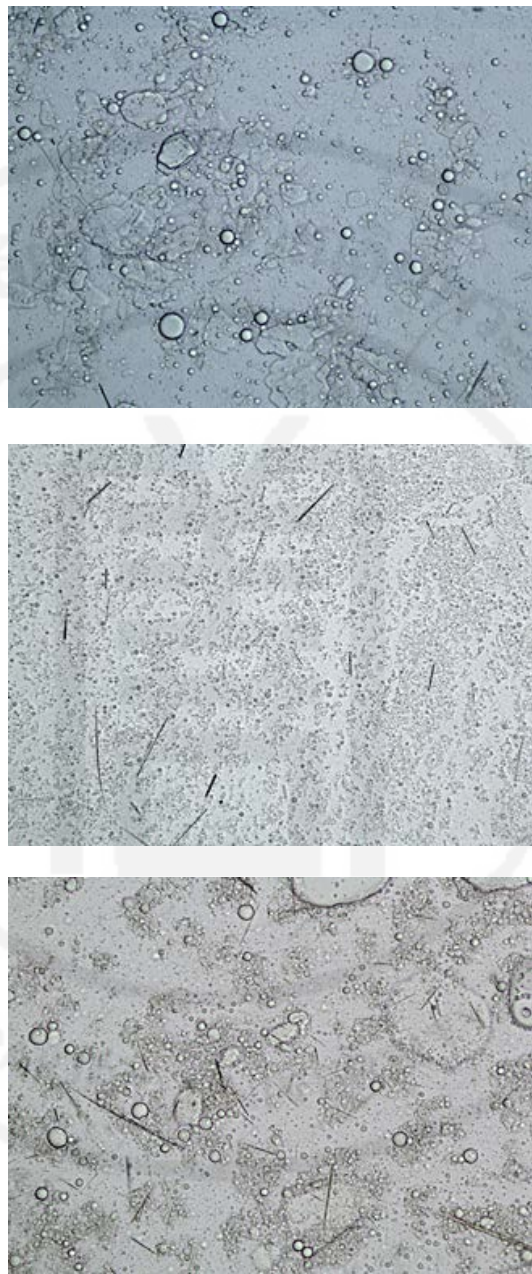
Figure 17 Optical micrographs (400x) of quercetin noisome dispersions prepared from Brij93:CHO at the molar ratio of 1:1 (upper), 2:1 (middle) and 3:1 (lower).
