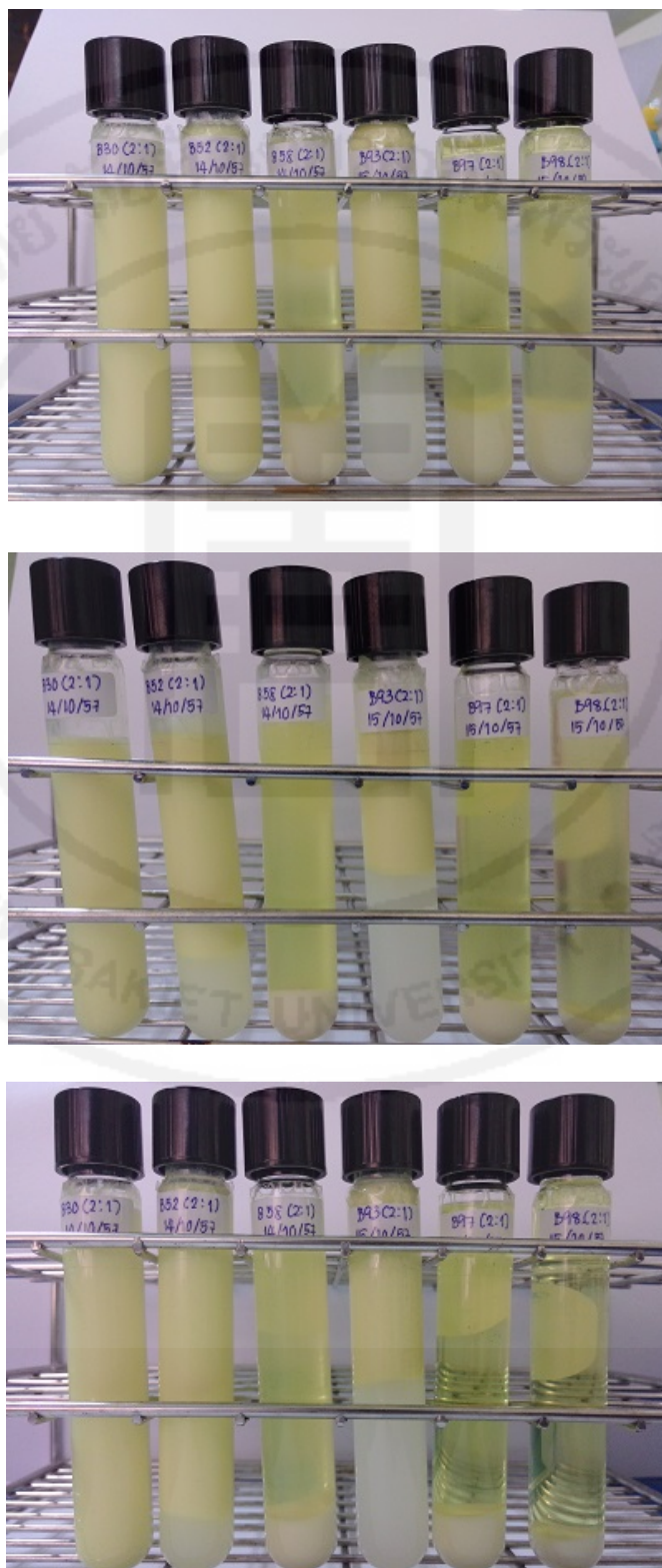
Figure 12 Photograph of quercetin niosome dispersions prepared from various non-ionic surfactants to cholesterol at 2:1 molar ratio after storage for 1 day (upper), 7 days (middle) and 30 days (lower)
